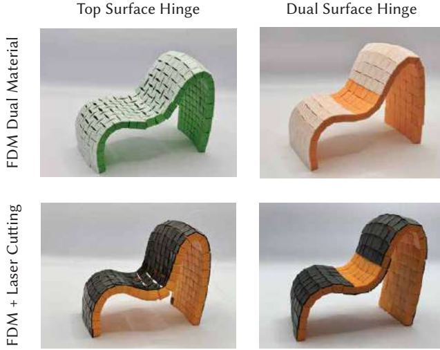
Fig. 14. Comparison of two fabrication methods and hinge placement strategies: Top: dual-material FDM printing with TPU linkages and PLA tiles. Bottom: laser-cut EPDM rubber hinges adhered to PLA tiles. Left: top-surface-only hinge placement. Right: hinges placed on the top or the bottom using the design optimization strategy presented in Section 4.4. Prototypes with dual surface hinge placement show improved quality over top surface only hinges.
