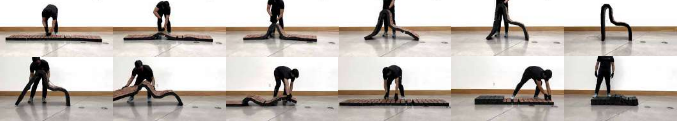
Fig. 13. Timelapse of deploying and disassembling a chair, demonstrating the reversible actuation capability of our method.
